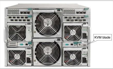
Figure 65: Position of the KVM blade
